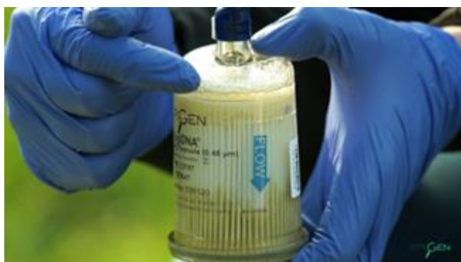
Figure 4. Illustration of the filtration capsule, with a total surface of 500 cm 2 allowing the filtration of 30 liters of water. Source: SPYGEN
