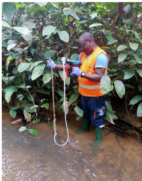
Figure 3. Example of sampling with a Vampire peristaltic pump provided by SPYGEN. Source: Terea
